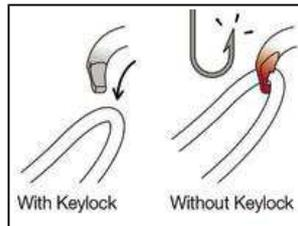
To ensure optimal efficiency, OK carabiners use the Keylock system: the body/gate interface does not have a hook that could snag on anchors, ropes, harness equipment loops...
