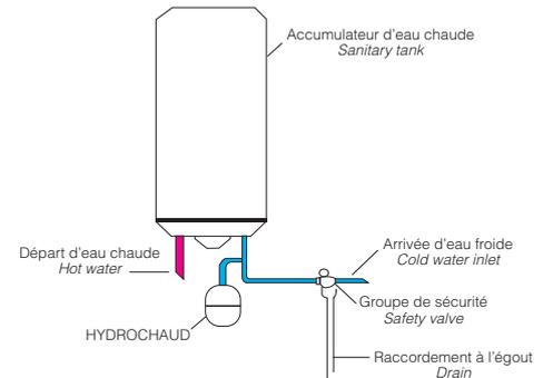
T°min/max: -10°C/+99°C - Pression max: 10 bar
