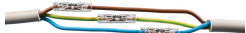
Strip 10 mm conductor per specification and insert connector (example shows staggered connectors).
