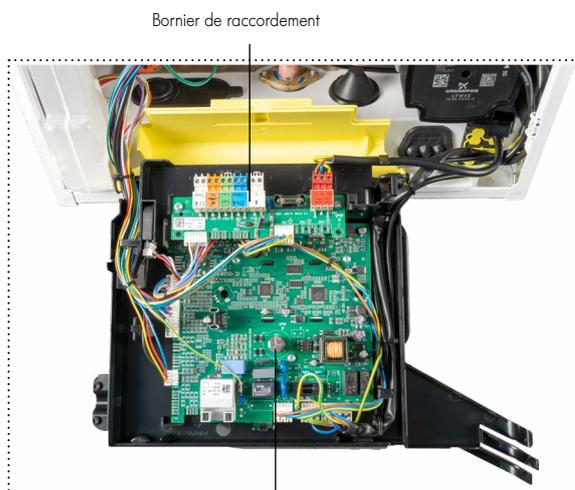
Bornier de raccordement
