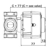
Installation dimensions for Actuator Series ARA600 with ESBE VRG100, VRG200, VRG300, VRB100 and VRH100 mixing valves
