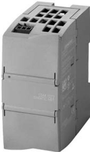
COMPACT SWITCH MODULE CSM 1277 RACCORD. SIMATIC S7-1200 ET JUSQ. 3 AUTRES PARTICIP. SUR IND. ETHERNET AV. 10/100 MBITS/S UNMANAGED SWITCH, 4 PORTS RJ45, ALIMENTATION EXT. 24V DC DIAGMOS.LED, MODULE S7-1200 AVEC GHB ELECTRONIQUES SUR CD
