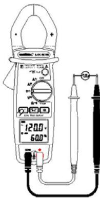
Position the switch on **V AC**, and press the **DISPLAY** key.
