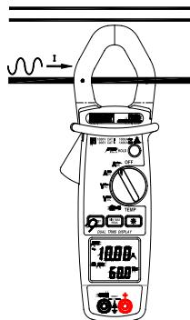
Position the switch on **A AC**, and press the **DISPLAY** key.
