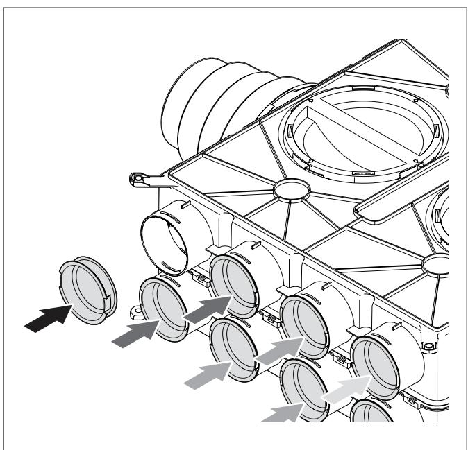
**EN** Connecting AE34C duct
