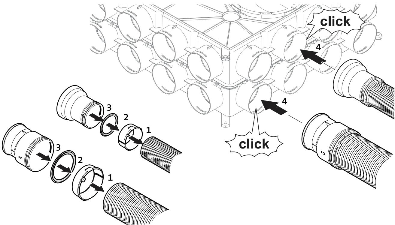
EN Connecting AE35SC / AE55SC duct
