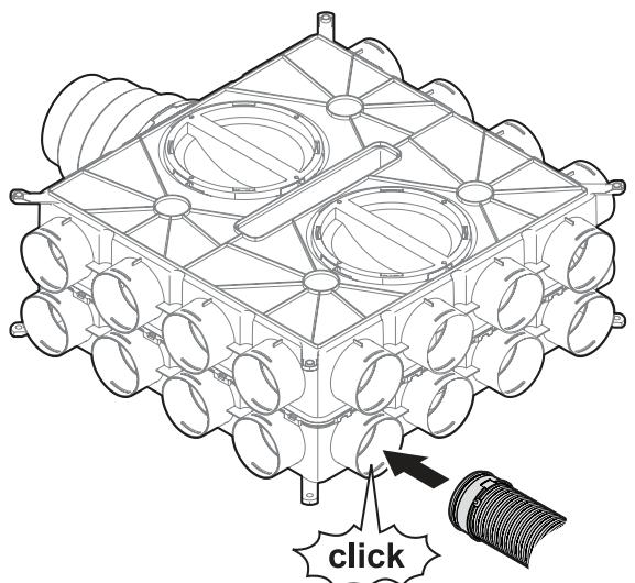
**EN** Connecting AE23C / AE48C duct
